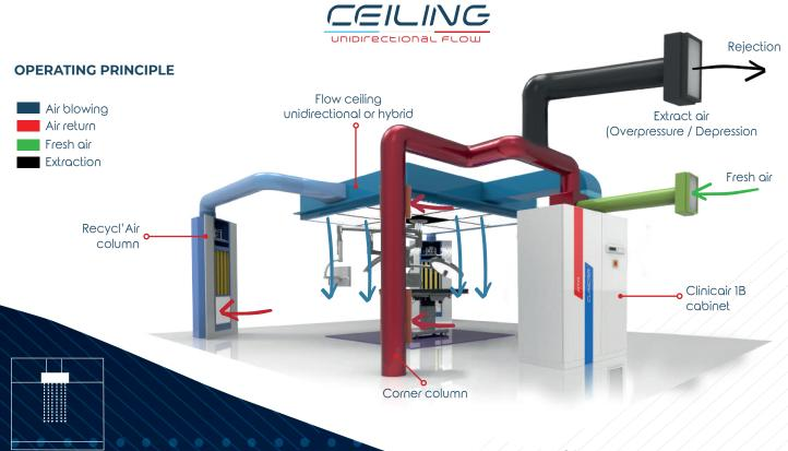
A unidirectional flow is a controlled air flow, having a regular speed and parallel air streams. This air flow regime results in the directed evacuation of particles from the clean zone (source: NF S 90-351 April 2013)
